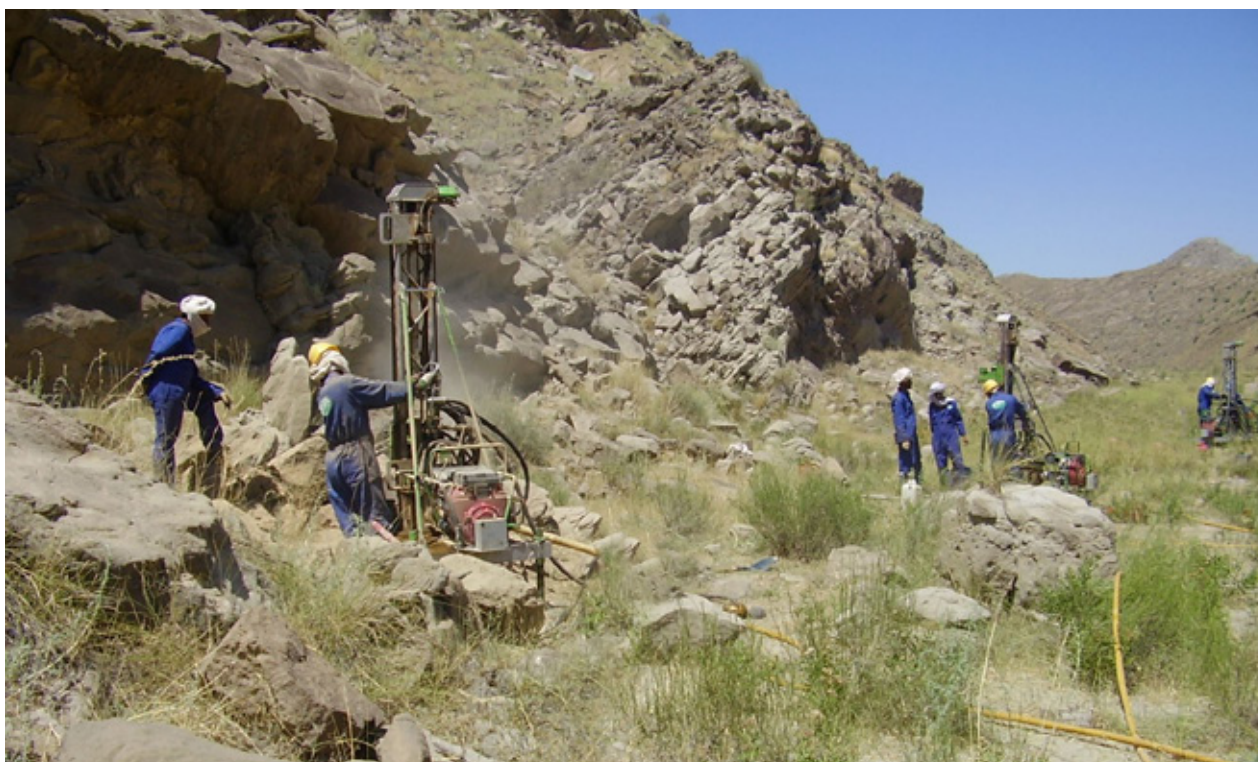
Hole drilling to load dynamite for seismic acquisition, district Karak, KPK.
