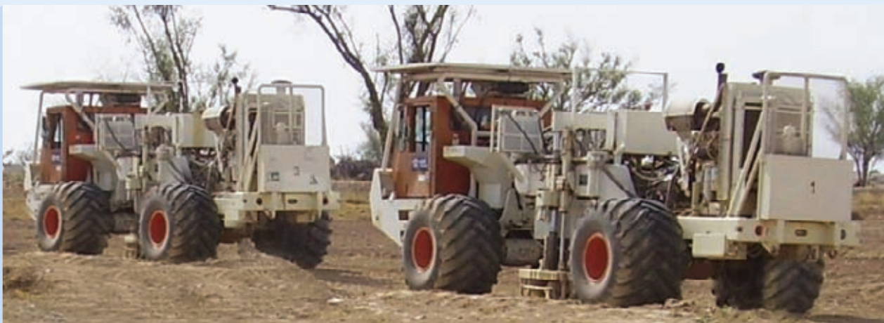
Seismic vibrators working for onshore hydrocarbon exploration.
