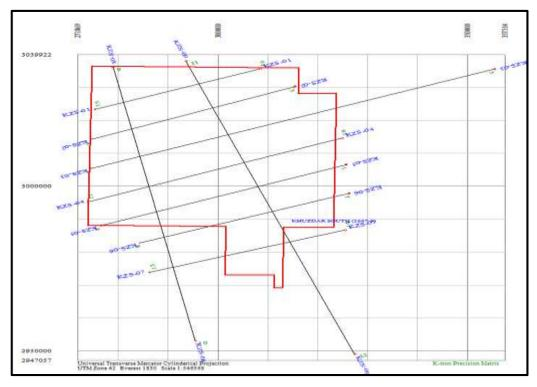
Orientation of strike lines can be changed after the acquisition of dip lines. The dip lines location can be changed subject to requirement.
