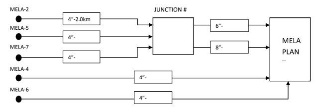
Due to rough terrain, elevation profiles, multiphase flow in pipelines and decreasing reservoir pressures of Mela field, significant pressure drop from wellhead to Plant has been observed which is impacting the overall hydrocarbon recovery from the field. To improve the hydrocarbon recoveries from the field, which is being impacted due to this surface network pressure drop, the Nashpa JV intend to evaluate and implement the cost-effective solution.
