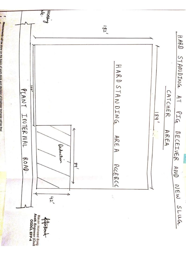
waster @ 6 c/c SECTION R.C.C SECTION P.C.C Man bas #4 HARD STANDING R.C.C (1:2:4) whto 6 depth P.C.C (1:2:4) upto 6 depth P.C.C. (1:4:8) who . 4 depth P.C.C. (1:4:8). where 4 depter SLu G A -I Soil Soil PIG CATCHER RECETVER AREA Distribution Bas # 4 @ 9" C/C long Bas Not according to scale. AND Hasan Waheed Baig Asstt. Engineer (Civil) OGDCL EFP-4 SEE
