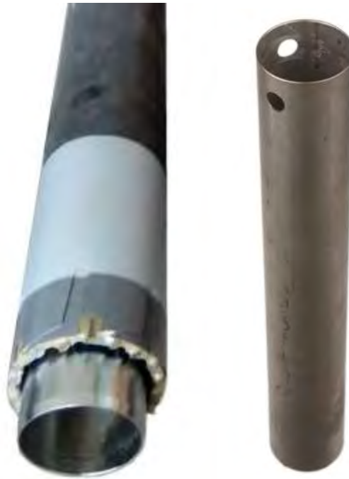
Figure 3.2 Double tube core barrel sampler and thin wall sampler
