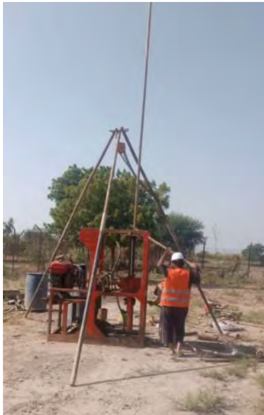
Figure 3.1 Straight rotary drilling machine
