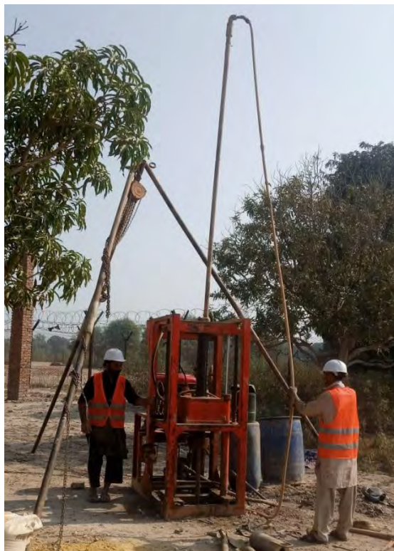
Figure 3.1 Straight rotary drilling machine
